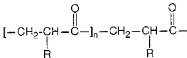
Where R may represent for example either H or CH<sub>3</sub>, POKETONE Polymer chains are flexible and possess the molecular symmetry and cohesive energy, derived from the perfectly alternating polyketone groups, necessary to produce a tough, high-melting-point, semi-crystalline thermoplastic suitable for a broad range of applications.
