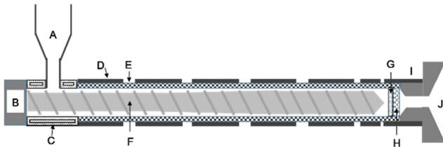
A: Hopper, B: Motor, C: Water cooling jacket,
