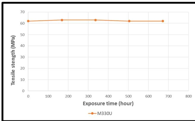
Figure 4.5.1.2 Influence of Weatherometer aging test(SAE J1960/2527) on the tensile elongation at break of 3.0 mm thick POKETONE Polymer M330U grade tensile test specimens
