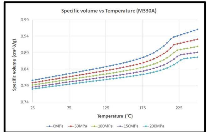
Figure 1.3.1.3 PVT curves for POKETONE Polymer M330A GF 30% Filled Compound (M33AG6A)
