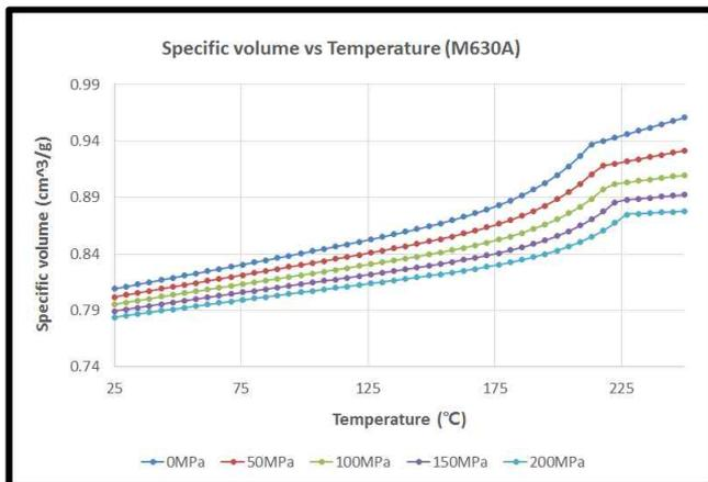
Figure 1.3.1.2 PVT curves for POKETONE Polymer M330A
