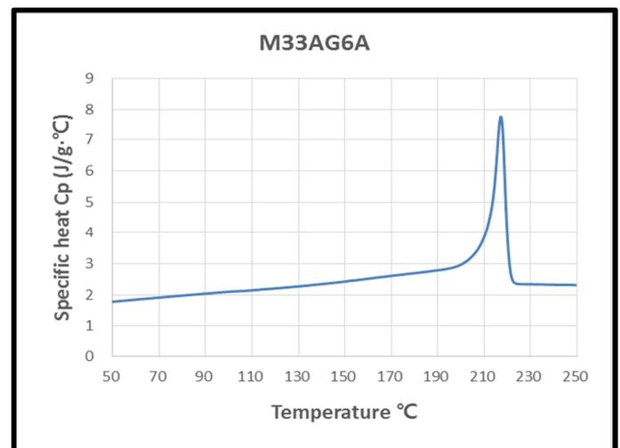
Figure 1.2.5 Specific heat capacity (M630A & M33AG6A)
